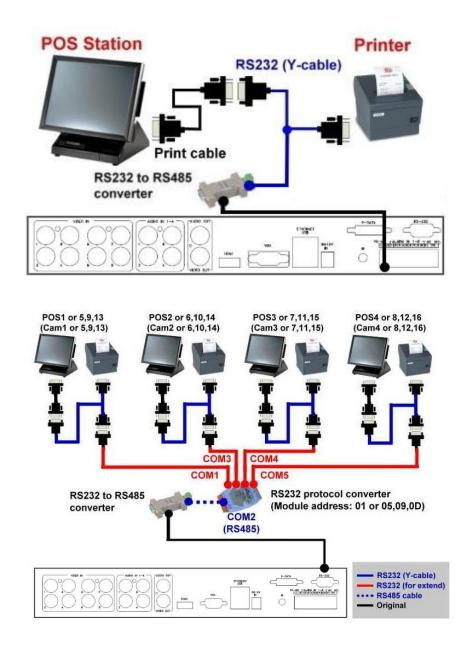
Top figure: 1-to-1; bottom figure: RS-232/Multiple, 1-to-many
