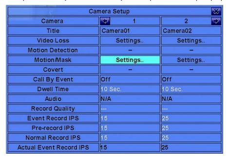
The Camera Setup allows the administrator to define the attributes for each camera. There are IP CAMs can be connected.
