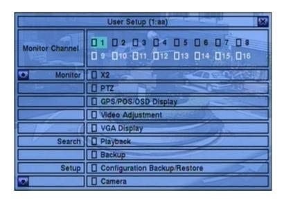
The Advanced User Setup allows the administrator to setup each user's detailed access right of the system.
