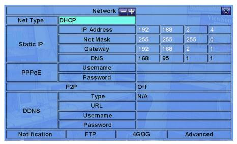
The Network Setup allows the administrator to setup all Ethernet network related parameters. Please check with your network administrator to set these parameters correctly.
