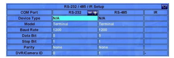
The RS-232/485/IR Setup allows the administrator to setup RS-232/RS-485 control port and NVR ID for IR remote. Please refer to the manuals for the connected devices - keyboard controllers – to set the items in RS-232/485 Setup.
