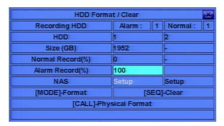
The HDD must be formatted before it can be used to record video/audio. The HDD Format/Clear screen allows the administrator to format and/or clear each HDD, and set the size for Alarm Record partition and Normal Record partition for each HDD. Please make sure there's no remote user before formatting the HDD.
