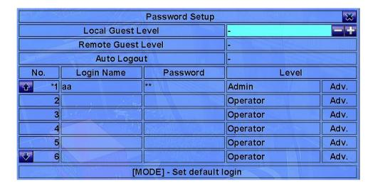
The Password Setup allows the administrator to add new users, delete existing ones, and/or modify the user's name, password, and/or level.
