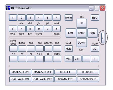
Please note that most of the buttons correspond to the keypads on the front panel. If you connect the PC through RS-232 and use an RS-232/RS-485 converter to connect to multiple DVR/NVRs, you would be able to control multiple DVR/NVRs via the simulation software. Please refer to <a href="Section 3.2 Optional Connections">Section 3.2 Optional Connections</a> to connect/cascade the DVR/NVR s to the PC.
