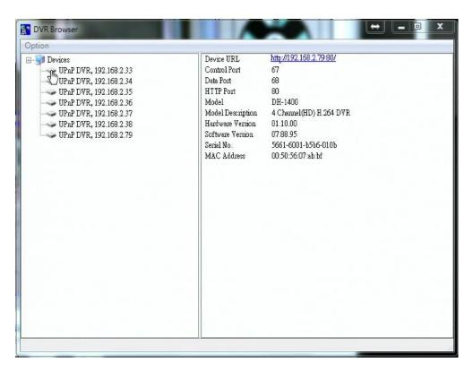
The utility will scan all the DVR/NVRs which support UPnP in the LAN. Please select the desired DVR/NVR device, and its detailed information will be shown on the right as above. Users can (1) click on the URL to call up IE and logon to the device, (2) select Option  $\rightarrow$  Rescan network, or (3) select Option  $\rightarrow$  Export Device List. The exported device list can be imported to IE software or CMS software in the future.
