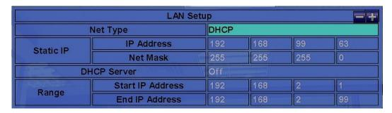
The LAN Setup allows the administrator to set LAN related parameters. Please note that the LAN is built in the optional POE module, and is used to interface with all IP-CAM which are connected through the IP-CAM (POE) ports. It has nothing to do with the Ethernet WAN port (labelled WAN).
