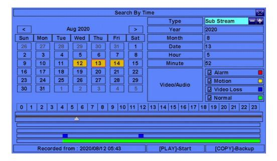
The Status field will show the 'Recorded from' time based on the selected Video/Audio before searching - alarm partition if any of Alarm, Motion, or Video Loss, is checked, and normal partition if Normal is checked. Above the status field is the 24H time slider and alarm/motion/video loss/normal recording status (from top to bottom).
