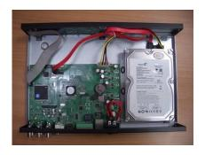
3. Hold the SATA HDD, and use a screwdriver to fix it as shown.
