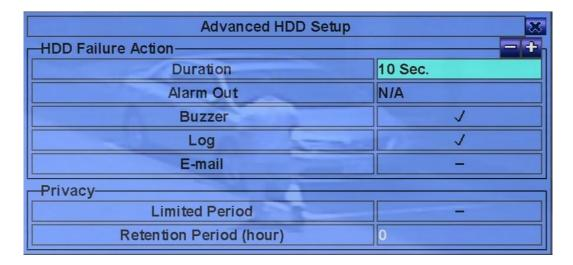
The HDD Failure Action in Advanced HDD Setup allows the administrator to define how the system responds to the detected HDD failure, while the Privacy settings allow the administrator to set the NVR to record for Limited Period and the Retention Period of its HDD storage. The HDD Failure Action will be triggered if there's no available formatted HDD detected.
