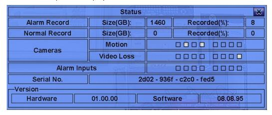
Status display includes Alarm Recording Status, Normal Recording Status, Camera Status, Alarm Input Status, Product Serial Number, and Product Version Number. Press **ESC** (Mouse: Right Click) to escape from Status display, and return to Menu display.
