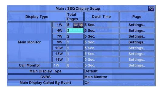
The Main/SEQ Display Setup allows the administrator to define the display pages in SEQ Display for main monitor and call monitor. Please note that Call Monitor supports 1/4 split window display.
