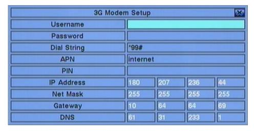
The 4G/3G Modem Setup allows the administrator to set 4G/3G modem related parameters if USB dongle 4G/3G modem is plugged in the USB port.
