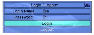
In Login/Logout display, follow the Text Input method described in Section 4.1 to enter the Login name and Password, press  $\blacktriangle \lor$  to highlight and select Login option, and then press ENTER to login the system. If the user wants to logout the system, just press  $\blacktriangle \lor$  to highlight and select Logout option, and then press ENTER. Press ESC to exit without making changes.
